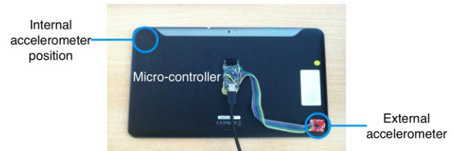
Figure 3. Test prototype with an external accelerometer.
